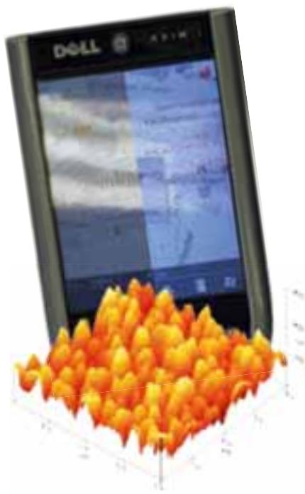
Display without anti-reflective coating (left) and with the moth's eye structure coating (right). AFM image of a moth's eye structure (front).
