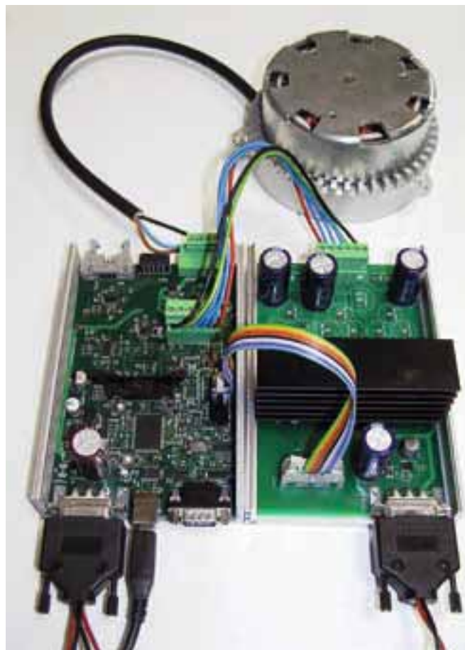
A control device for BLDC engines with a control circuit board (left) and a power board
