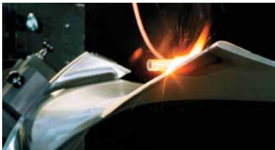
Depth hardness solution annealing with a laser
