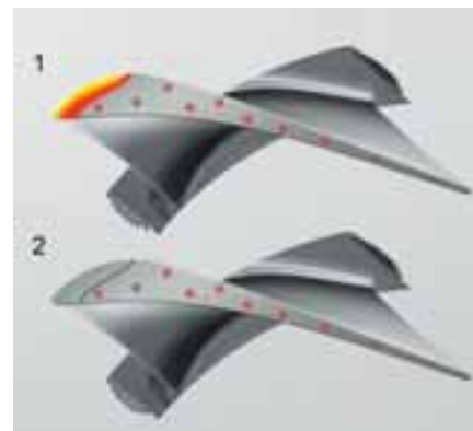
Separation of Cu precipitations (1) and Precipitation of fine Cu clusters (2) on leading edges exposed to greater wear and tear
