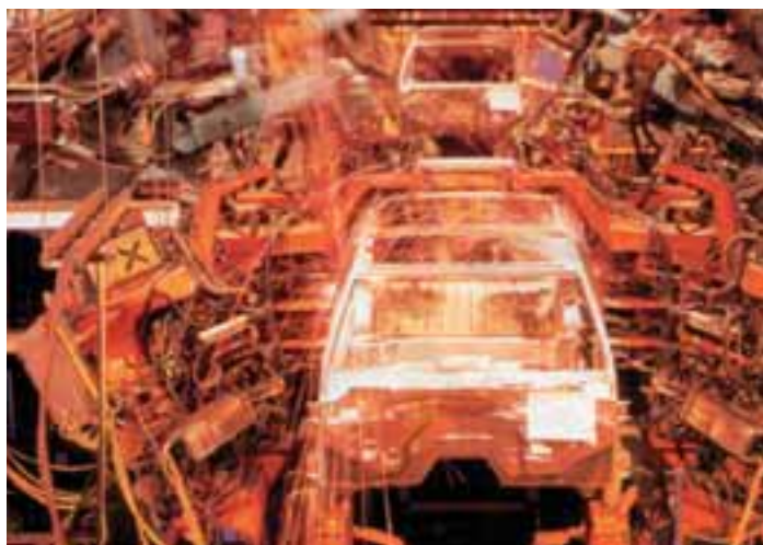
Resistance welding processes in the automotive industry, © Harms & Wende GmbH
